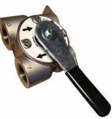
If you have a brass bypass, like the example on the right, turn the handle to move the notch on the top of the bypass from service to bypass following the directional arrows. This shuts the water off to the softener while allowing the rest of the residence to have water (untreated).
