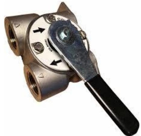
If you have a brass bypass, like the example on the right, turn the handle to move the notch on the top of the bypass from service to bypass following the directional arrows. This shuts the water off to the softener while allowing the rest of the residence to have water (untreated).
