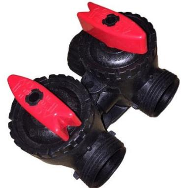
1. Normal Operation Position: The inlet and outlet handles point in the direction of flow indicated by the engraved arrows on the control valve. Water flows through the control valve for normal operation of a water softener or filter. During the regeneration cycle, this position provides regeneration water to the unit, while also providing untreated water to the distribution system. (See Figure 1)
